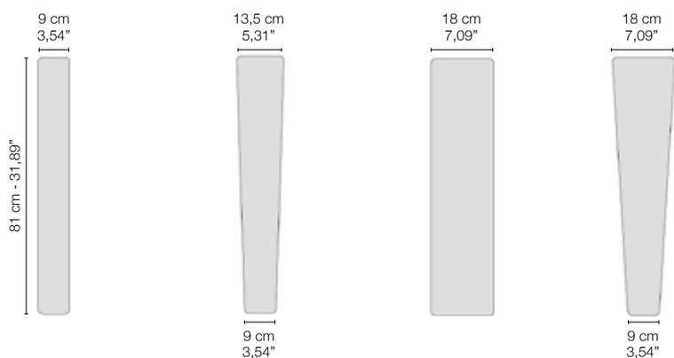
dimensions may vary due to leather, foam thickness and density, covering materials and position of reclining mechanism. Allow for small deviations - especially for row configurations
